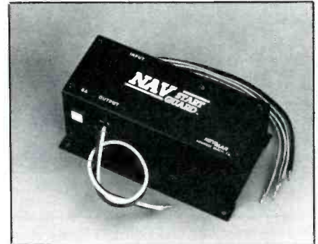
This device "floats" your radio equipment to prevent a memory dump during engine cranking.
