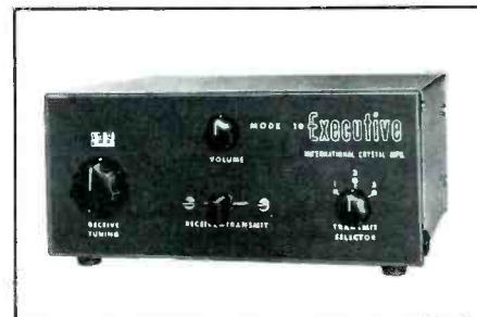
International Crystal produced the no-frills 3-channel "Executive 10" about thirty years ago. Not a bad little rig.
